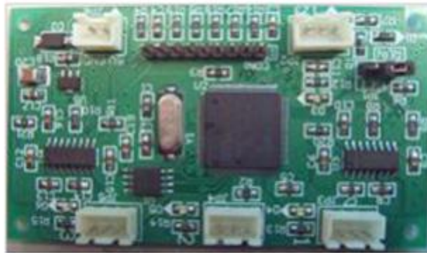
Multiple serial port multiplexing module
