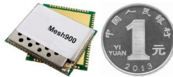
Mesh900-1Watts Module(Weights only 5 grams!) 26.5x33x3.5mm
