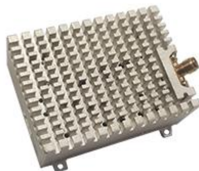
3 W: COFDM Ground low delay CVBS transmitter above 3 km (6.7x4.8x2.3cm,80g)
