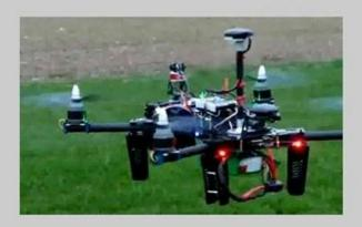
Integrated backup system for in-flight recovery and manual override with a dedicated processor and stand-alone power supply
