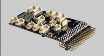
14 PWM/servo outputs (8 with failsafe and manual override, 6 auxiliaries, high-power compatible)
