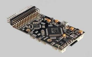
Advanced 32 bit ARM Cortex® M4 Processor running NuttX RTOS
