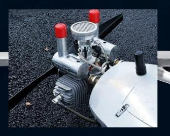
The DLA starter-integrated engine adds a starter and a generator motor. Starting and generating electricity are completed by the same brushless motor.
