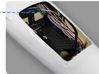
Device compartment: 16 \times 20 \times 8\text{cm}
