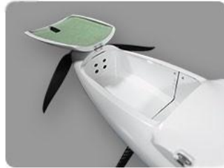
Battery compartment: 20 \times 9 \times 6\text{cm}
