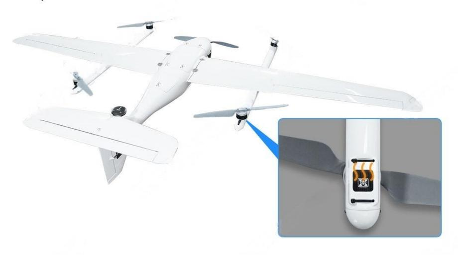
It supports multiple mapping payloads: orthographic cameras, 5 lens oblique camera, hyperspectral cameras, multispectral cameras.
