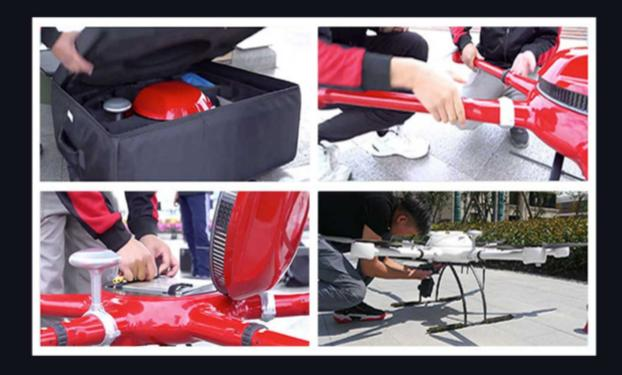
The plug-in arm design realizes quick disassembly and assembly, reduces the packaging size, and is easy to carry
