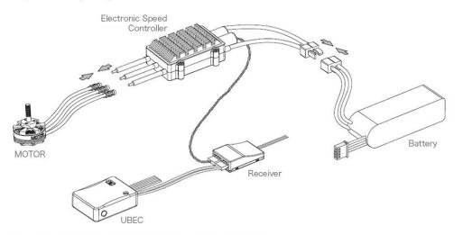
▲ For safety sake, please remove the propellers during throttle calibration!
